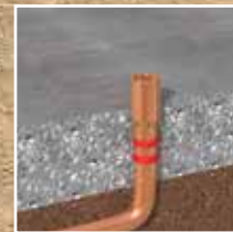
Sealing of penetrations
