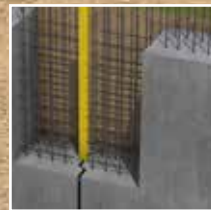
Connection joint with aof diaphragm wall
